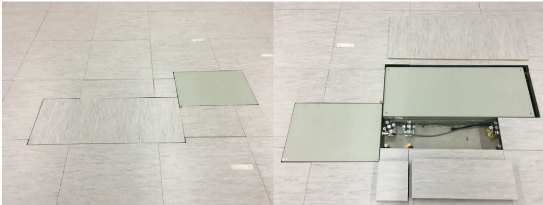
Fig. B.4: Detailed view of the force platforms; left: with the leveling covers; right: without the leveling covers.
