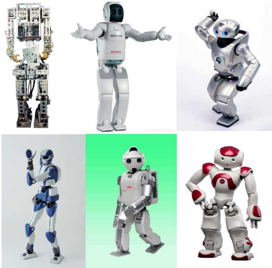
Fig. 2.11: Examples of humanoids robots developed throughout the world: WABOT-1, ASIMO and QRIO (top from left to right); HRP, HOAP and NAO (bottom from left to right).
