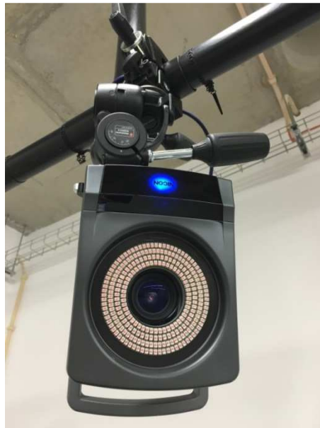
Fig. B.3: Detailed view of one of the infrared cameras, model MX T-20S.
